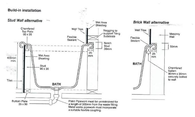
Due to its exceptional rigidity, this pressed steel bath requires rim support only. No mortar bed is necessary. However, to avoid flexing of the bath when used, mortar bed is reccomended.
